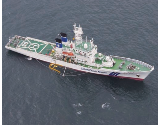
Oil spill skimming drill
