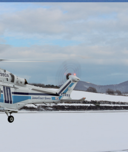
MH Eurocopter EC225 helicopter Length overall : 19.50meters Height : 4.97meters
