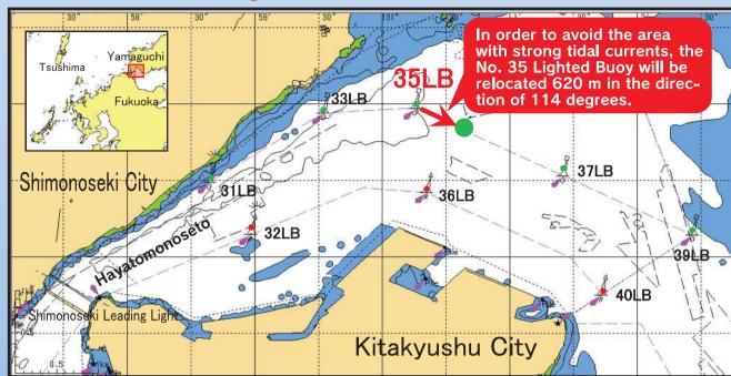
The Kanmon Route No. 35 Lighted Buoy, which has been located in an area with strong eastward tidal currents, causes vessels to converge and often hit the buoy. The lighted buoy will be relocated to a new position to prevent the buoy from being damaged or moved. Please note that there will be no object at the old position after the lighted buoy is relocated.
